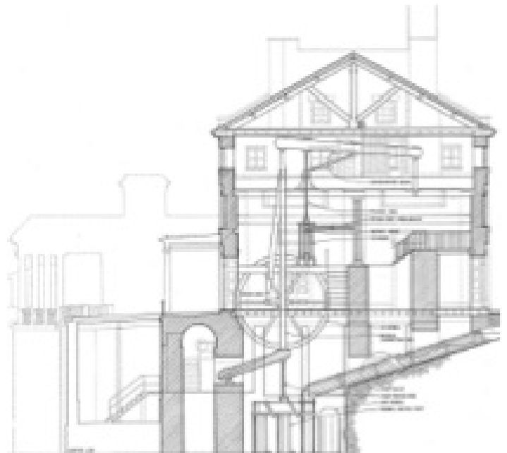
6.2.2 North Engine, Fairmount Waterworks (Courtesy of Historic American Engineering Record, U.S. Department of the Interior)
