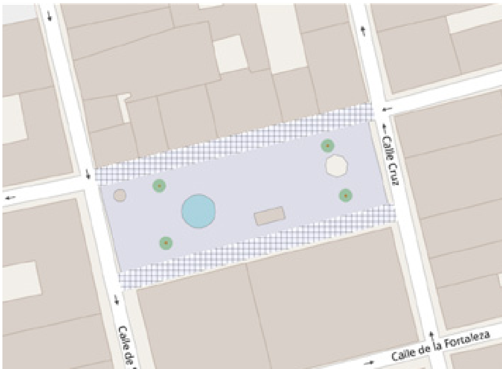
Figure 59: Existing conditions (top) recommended changes (bottom) to Plaza de Armas. Partially pedestrianized streets are hatched, while fully pedestrianized streets are in blue Source: Apollon and Nguyen. (All base maps come from openstreetmap.org, edited by the authors).
