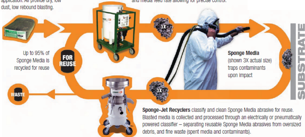
Figure 6.1.2. Illustration of Sponge-Jet® system, 2009. Credit: www.spongjet.com
