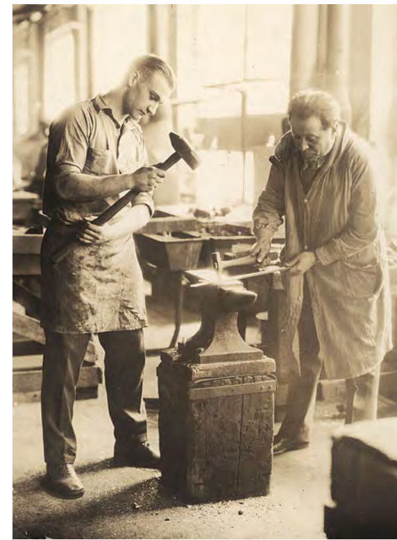
Figure 1 Yellin working at the anvil with a striker, 1920s. work and robustness of design.” 19 Today Clare Yellin, Samuel Yellin’s granddaughter runs the shop. As the designer and business person, she oversees the company’s two ironworkers who operate out of a forge in Chester County. With access to such extensive records, Clare has been able to restore thousands of works originally created by her grandfather. The family also donated over 2,343 original drawings by Yellin to the University of Pennsylvania Architectural Archives in remembrance of the greatest ironworker, Samuel Yellin. 20
