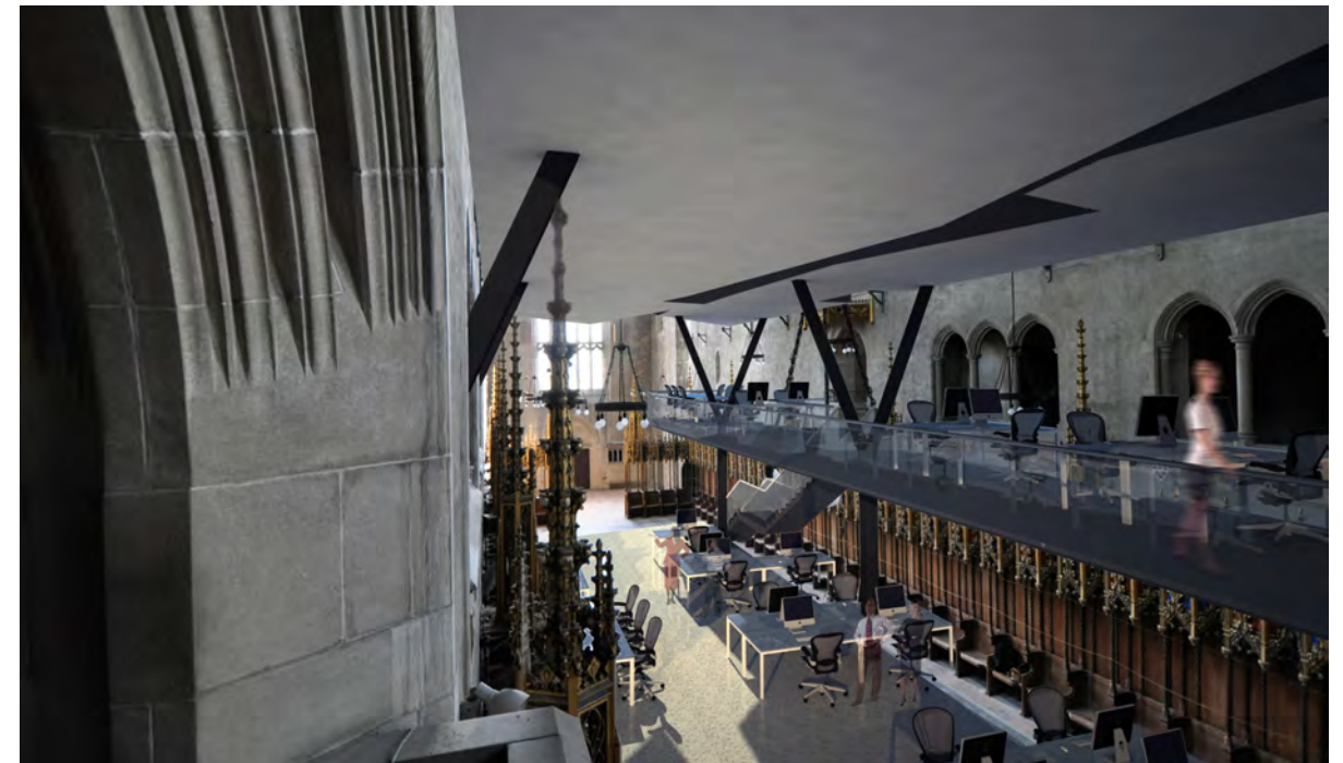
Figure 18 Rendered view looking southwest, showing mezzanine (red in diagram) beneath plate 2 (blue). Columns come to a Y to protect the west choir stalls.
