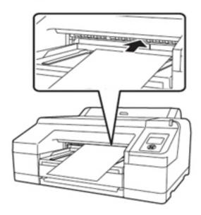
5. Push the paper under the gray feed rollers inside the printer.
