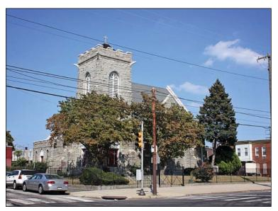
The building exterior is in good condition, some cracking and separation of the mortar from the granite is apparent. A large ivy vine is covering the one of the east walls, growing behind the fenced in air-conditioning unit.
