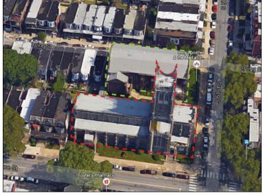
The property has two buildings connected by a hyphen at the first story. The primary building has a cruciform design, schist exterior walls, and limestone trim. The buildings are surrounded by small grassy areas and planting beds, with hedges and some chain-link fencing around the perimeter of the property. The site is well maintained.
