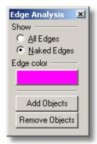
The naked edges display in the **Edge color**. These edges have gaps. The command line displays the number of open edges.
