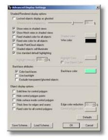
Mesh faces have a front and a back. The front direction is called the *normal* of the face. Some STL meshes need to have consistent normals to work correctly. By default, the front of a face is colored the layer or object color. When you run Rhino is shaded mode, you can show the mesh edges and color the backs of the mesh faces a different color than the fronts of the faces. This provides a quick check of face normal direction.
