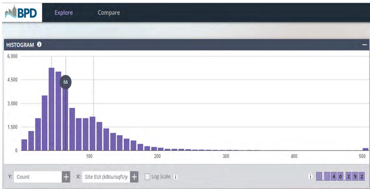
Figure 24- Example of building energy consumption distribution from Building Performance Database
