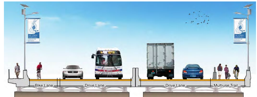
Proposed improvements to the Grays Ferry bridge, enhancing pedestrian and bike access
