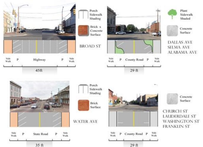
Figure 2.46 : Road Condition in Downtown
