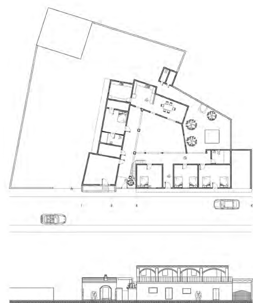
Figure 14. Plan and elevation of the Robles mother's remittance house. Note the awkwardly shaped living room just off the street, the two adjacent kitchens in the rear left corner, multiple bedrooms, two indoor bathrooms, and two outdoor bathrooms. Courtesy of Job Daniel Robles Robles.
