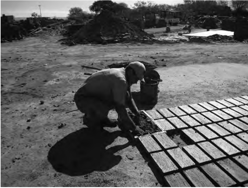
Figure 12. This is one of Autlán's largest brickyards. All the bricks are made by hand without shelter from the sun. Photograph by author.
