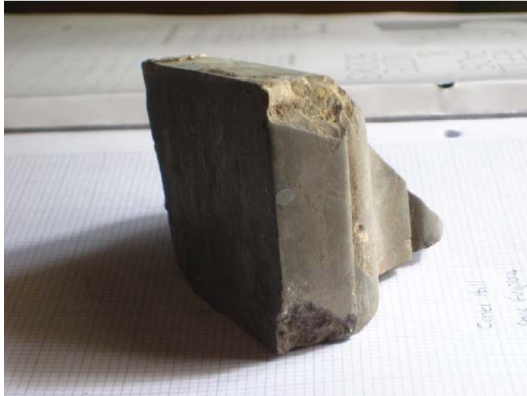
Figure I.45: Fragment of the original mitered corner piece of the dog-eared marble fireplace surround. Source: University of Pennsylvania.
