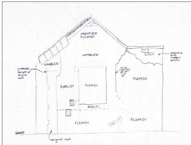
Figure II.5: Illustration of the different brick bond work on the west wall. Note the consistent Flemish bond along the bottom portion of the wall. Solid lines indicate obvious seams. Dashed lines indicate less obvious seams. Slashed lines delineate the boundaries of the brick work. Source: University of Pennsylvania.
