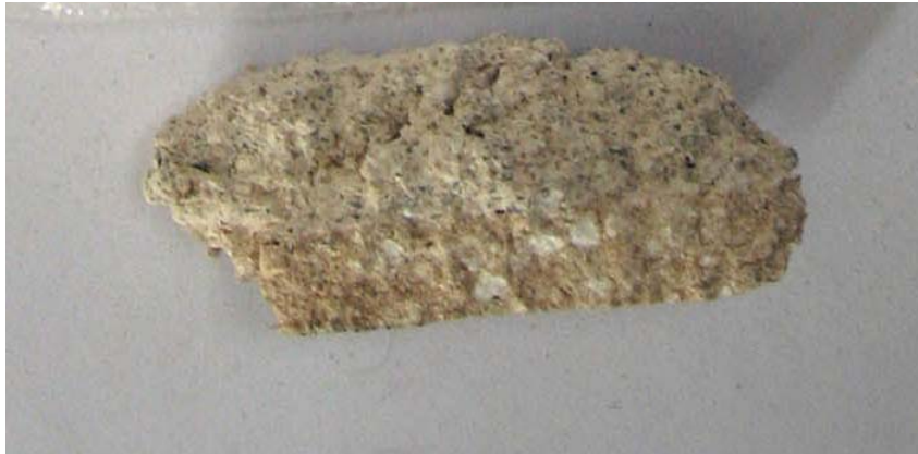
Figure P7: Photograph of Sample 19 depicting typical consistency of stucco from the first campaign. Source: University of Pennsylvania.
