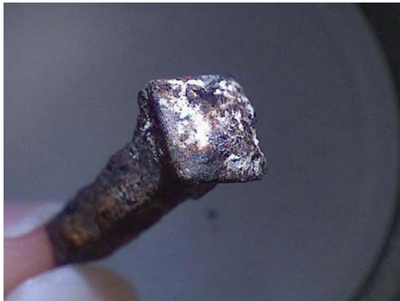
Figure III.10: Cast iron nails often had square heads, a detail that would not be possible with hand-wrought metal. Source: University of Pennsylvania.
