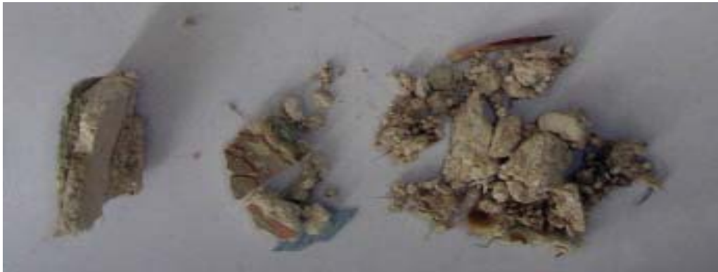
Figure P2: Photograph of Sample 10 depicting typical consistency of plaster within Campaign B. Source: University of Pennsylvania.
