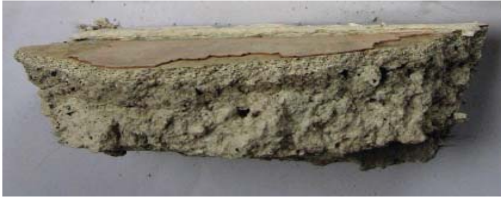
Figure P4: Photograph of Sample 33 depicting typical consistency of plaster within Campaign D. Source: University of Pennsylvania.
