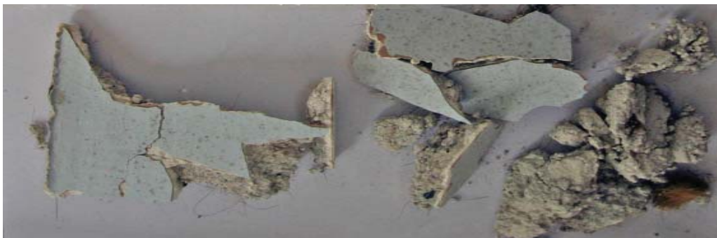
Figure P3: Photograph of Sample 11 depicting typical consistency of plaster within Campaign C. Source: University of Pennsylvania.
