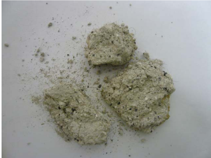
Figure III.5: The plaster from the octagonal room walls and the apse are identical and are thought to be of the same campaign. Note the black inclusions, use of hair, and the same gray color. Source: University of Pennsylvania.
