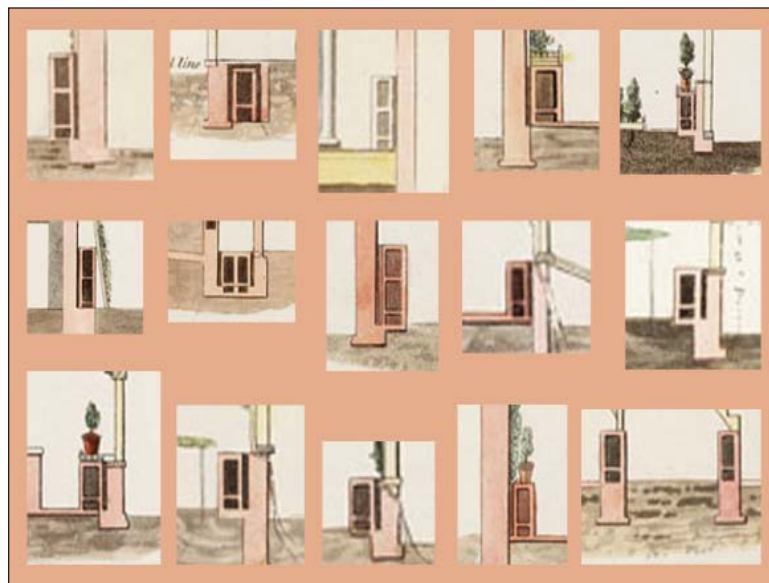
Figure 60: Examples of flue systems from Tod's Plans, elevations and sections, of hot-houses, green-hous-es, an aquarium, conservatories, &c., recently built in different parts of England, showing independent rear flues with larger upper chambers. Source: English Heritage.
