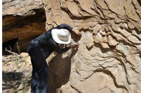
Rilem Test, Holly Tower, 2013
