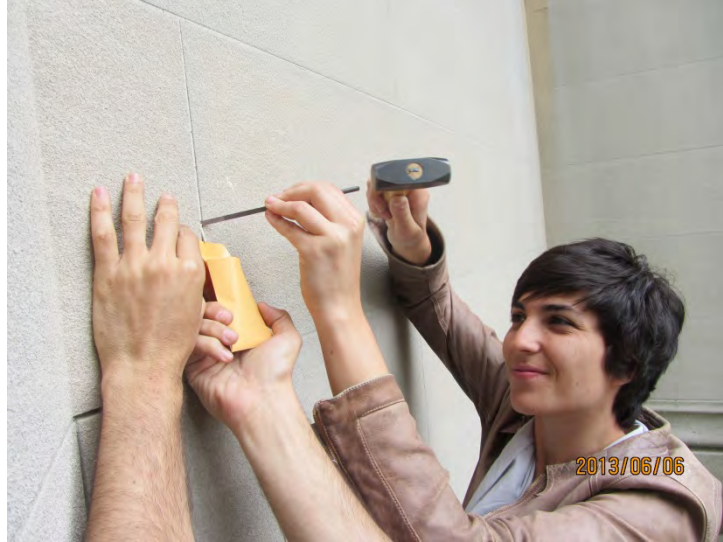
Sampling the Exterior Masonry Wall, 2013
