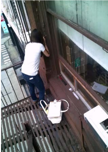
Taking paint samples from a cast iron building, 2015
