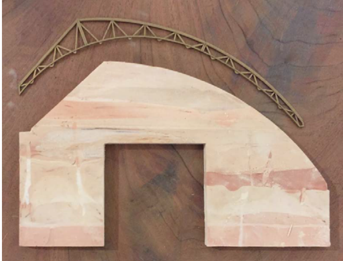
Stamped earth wall and truss of greenhouse model, August 2016.
