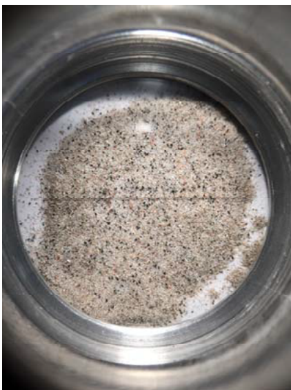
Figures 1 & 2: Acid Digested Mortar Sample; Galt Post Office Mortar Analysis: Cambridge, Ontario.
