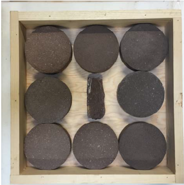
Figures 3 & 4: Prepared Samples of Composite Patches for Brown Stone & Building Archaeological Investigation of Mouldings at 2041 Delancey Street, Philadelphia.
