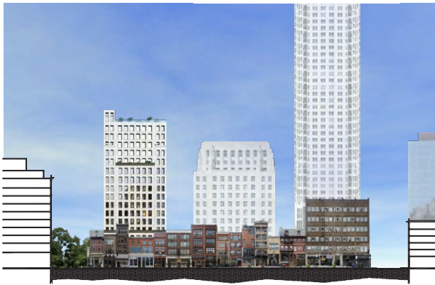
White Toll Bros. Tower - 16 Stories with facadectomy
