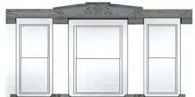
Figure 6: Third story stone window surround engraved.
