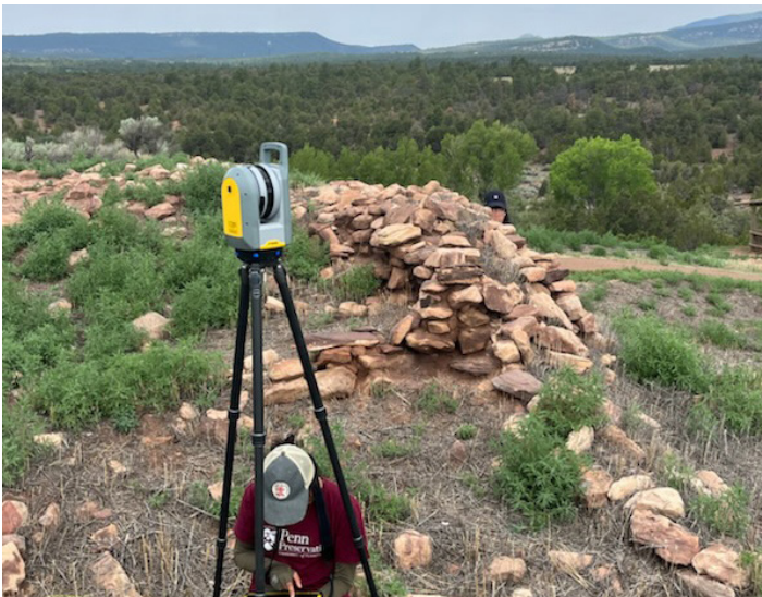
Image 1 (left): Operating the Trimble X7 laser scanner to capture the northern exterior wall of Pecos Pueblo in the three-dimensional model of the site.
