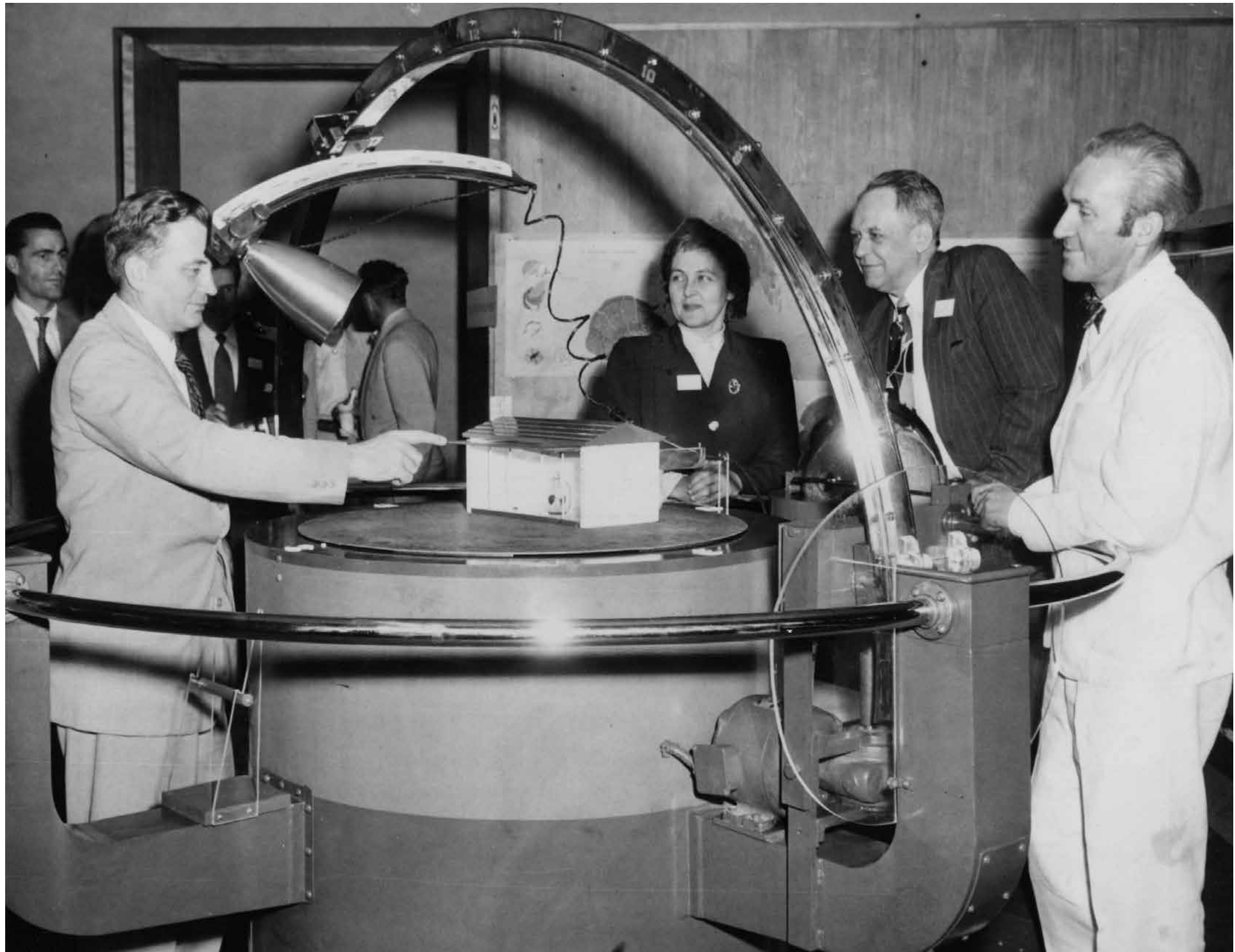
11; "The Solarometer, which can depict the angle at which the sun will shine on any house in North America at any given time, being discussed at the M.I.T. Symposium on Space Heating with Solar Energy; left to right: Professor Lawrence B. Anderson, symposium chairman; Dr. Maria Telkes, owner of the solar house in Dover; Dr. W.J. Arner of Libby-Owens-Ford Glass Co.; and George Fred Keck, Chicago Architect." August 1950, by Maynard White. M.I.T. Historical Collections.
