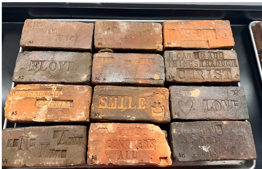
Image 1: The samples given to the ACL by the Baltimore Community Brick Project for compression analysis.
