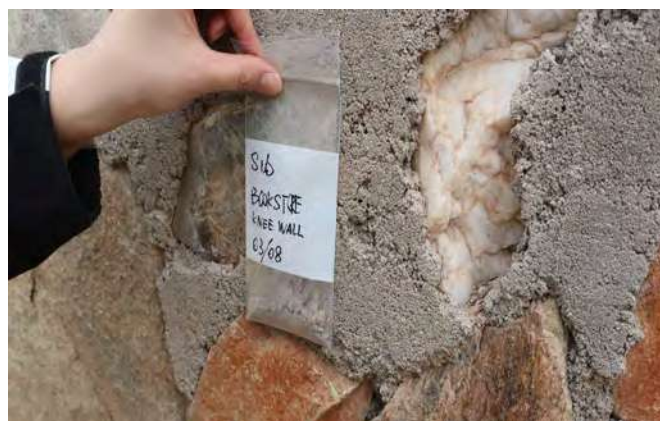
Figure 3.12. Collecting concrete samples from less visible areas at Taliesin West. (Source: taken by authors)
