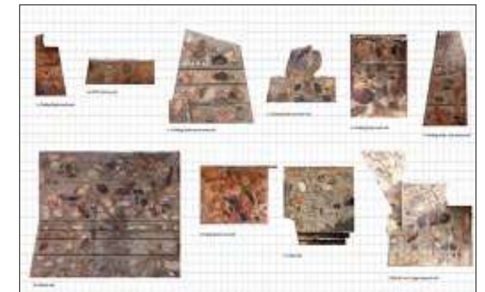
Figure 3.14. Orthoimages of each survey area exported from point cloud models in Agisoft and organized by periods. (Source: created by authors)
