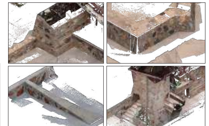
Figure 3.16. Isometric images of each survey area exported from point cloud models in Agisoft. (Source: created by authors)
