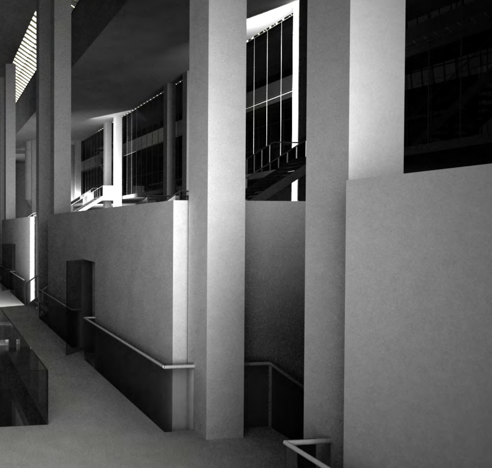
Image 10.5.30- Adaptation of the boiler house, which takes advantage of the skylights above and maintains the feeling that the existing stairways and catwalks provide, while opening them up to the space below to allow natural light to penetrate down to the ground floor. Peter Hiller
