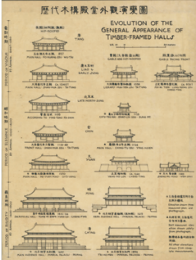
历代木构殿堂外观演变图，梁思成，1930年代 Evolution of the General Appearance of Timber-framed Halls, Liang Sicheng, 1930s
